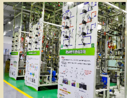
Catalyst performance testing equipment
