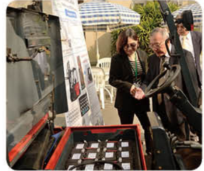
Electric stacker with LTO energy storage system
