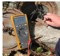
Cathodic protection Anti-corrosion by cathodic protection
